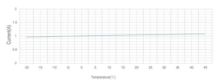
Note: This curve is test data of 1M LED Strip.
