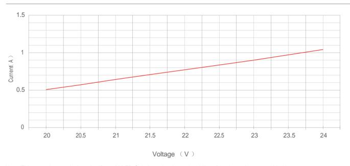
Note: This curve is tested when the IP20 1M LED Strip is under thermal stability after 2h continuous working in 15°C room temperature.
